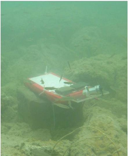
Figure 3: Example of Periphyton sampler
